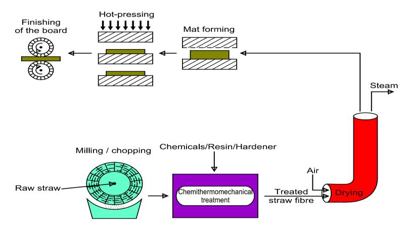
FIGURE 1. Schematic diagram of the strawboard production incorporating the new process.
