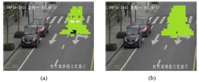
Fig. 6. (a) A car detected in a traffic video. Note the macroblocks of zero motion vector on the object's surface. (b) Correction by painting the whole car as a rigid object through morphological dilation.
