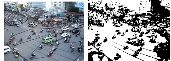
Fig. 5. Hanoi cross road group of cars, group of tracks and thresholding [4, 5]; temporal window should not be too small nor the detection threshold too high; the images are further eroded or dilated to form the traffic areas within the crossroad.
